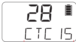
CTCSS is enabled and set to tone 15 (107.2 Hz)
