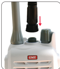
2. INSERT THE CHARGER PLUG
