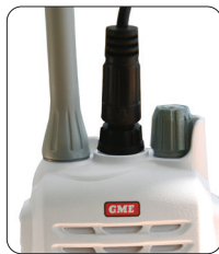
3. ROTATE THE COLLAR TO SECURE THE PLUG
