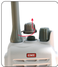
1. UNSCREW THE CONNECTOR CAP
