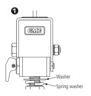
To assemble the fold down antenna mount, ensure that the washer and spring washer are positioned properly.
