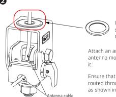
Insert spacer ring to suit antenna with a 1/2" mounting stud.
