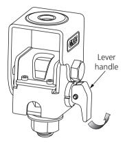
Pull the lever handle out to retract the locking pin. Fold the antenna to the desired position. Engage the locking pin with the closest locking hole position. Release the lever handle to lock the antenna mount position.
