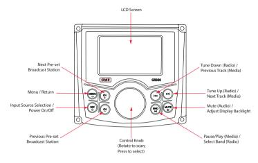
The diagram below details the operational controls of the GR350BT radio.
