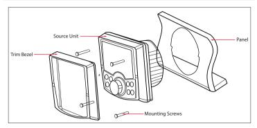
**NOTE:** Select a suitable mounting location. Then examine the area behind the panel to determine if there is sufficient access for routing the cables and fitting the mounting screws. For panels of 6 - 9 mm thickness such as aluminium, plywood or fibreglass, the unit can be mounted using the 12 mm screws supplied (refer the diagram above).
