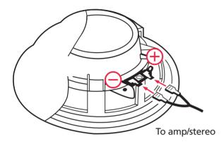
Remove the speaker grille (turn anti-clockwise). Fit the speaker into the cutout and secure the speaker using the screws (supplied).
