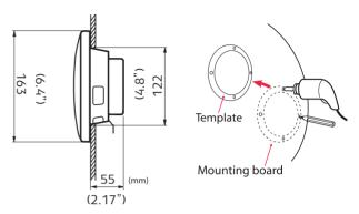
Use the template supplied to mark the position of the mounting screws and the outline of the speaker hole. Drill the mounting holes using a 3.3 mm drill bit and cut the hole for the speaker.
