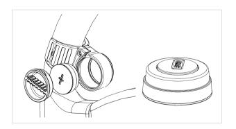
6. Use a 10c coin OR a Flat head screw driver (max size 1.2x6.5mm). Do not use other tools as it might damage the slots.
