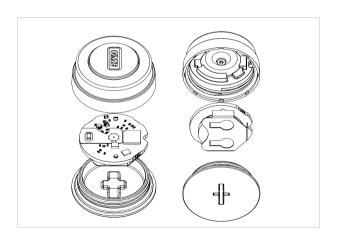
8. Remove and Replace 3V CR2032 coin cell battery.
