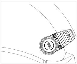
Use 2.5mm Hex key to hand tighten (do not over torque or use a power driver) two bolts to clamp down the mount. The mount is designed to fit a variety of steering wheel diameters as shown below:
