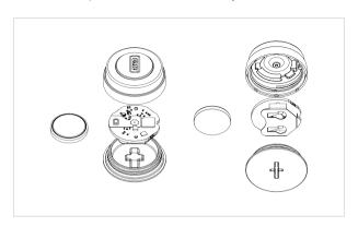
9. Place PCB with new coin cell into main housing. Use the orientation notch to align pcb in correct position.
