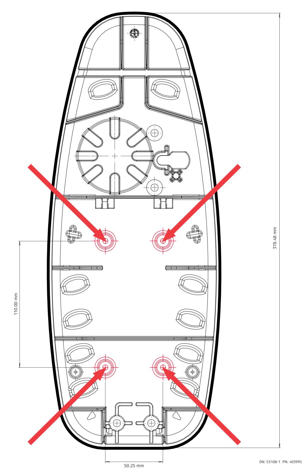
Provide 700 x 300 x 300 mm of unobstructed space for the installation of the Float-Free housing.
