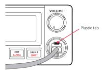
Gently press the rubber strain relief grommet into the hole surrounding the socket so that the slot around the grommet fits neatly inside the lip inside the hole.
