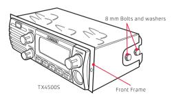
4. Secure the radio using the four 8mm bolts supplied.
