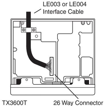
For details on connecting the TX3600T to a CIU or a PC or for general installation options and tips, refer to the Telemetry System Manual P/N 310181.
