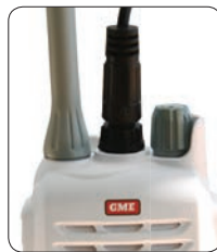
3. ROTATE THE COLLAR TO SECURE THE PLUG
